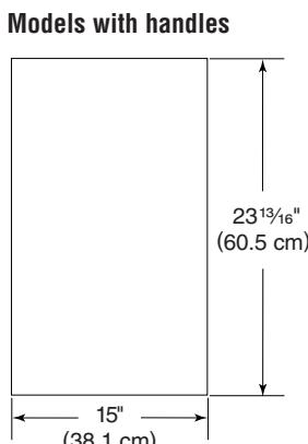
Panel should be 1/2 to 5/8 in. (13 to 16 mm) thick. NOTE: A thicker panel may need rounded front corners and a cutout for access to the handle.
