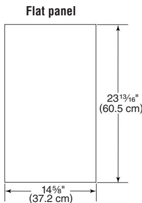
A 7/32 in. (5.6 mm) thick panel is required. This is the same thickness as a standard 1/4 in. plywood or paneling.
