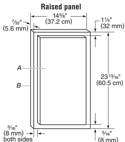
The outer section of panel must be 7/32 in. (5.6 mm) thick to fit into trim. Design raised panel sections using dimensions shown above.
