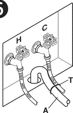
NOTE: If longer drain hose is required, order drain hose extension kit, GE part number WH49X301. Connect additional drain hose (contained in kit) to original hose with hose clamp (contained in kit).
