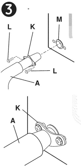
**3** Connect drain hose **A** to drain opening on back of washer. Push hose **A** into opening using your hands until clamp **K** on drain hose is about 1/2" from washer back. Insert 2 screws **L** through holes in clamp **K** and into holes at either side of drain opening. Tighten screws with screwdriver or 1/4" nut driver. Clamp **K** will be bowed and about 1/4" from washer back after screws are tightened.
