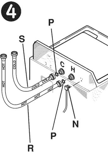
**4** Remove electrical cord **N** from storage before installing water hoses. If not installed, install rubber washer **P** in one end of hot water hose **R**. Thread hot water hose **R** onto connection labeled **H** at top rear of washer. Hand tighten, plus an additional 1/8 turn with pliers.
