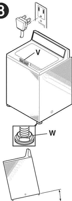
Make sure large dial control on washer is pushed in to the OFF position.
