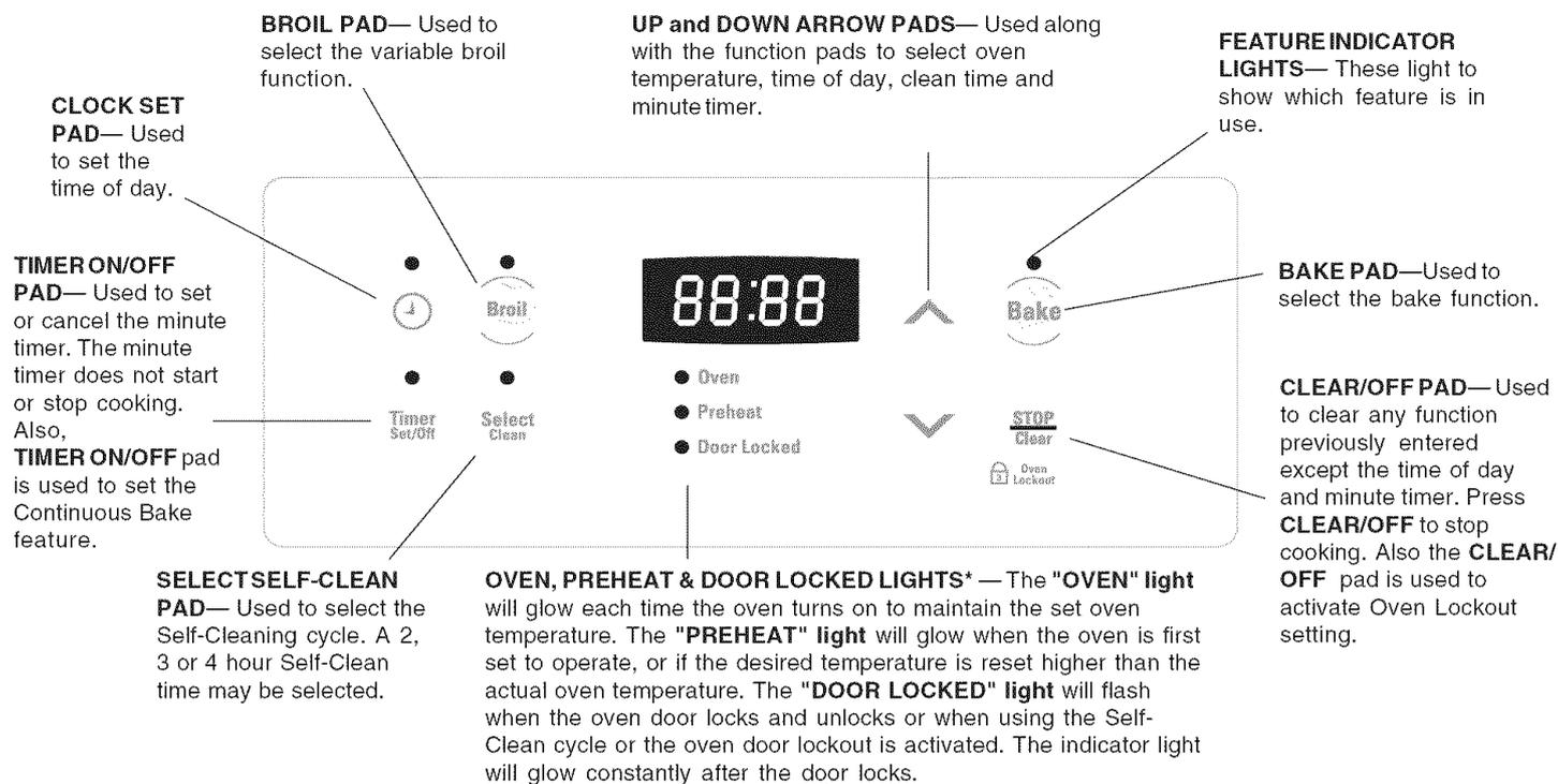
\*Note: The **OVEN** indicator light on the electronic display will turn ON and OFF when using the Bake feature and during preheat. This is normal and indicates that the oven is cycling to maintain the selected baking temperature. When the preheat indicator light turns OFF, your oven is ready.
