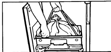
4. Remove bag carrier handles from side retainers and hold. **For easy bag removal**, release side of drawer by opening the latch at the right front. Lift bag and carrier out of drawer.
