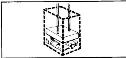
The compacting ram does not go to the drawer bottom. You will not see compacting of the first few loadings.
