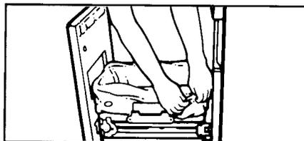
5. Lock bag in place by tucking cuffs behind bag retainer and by pulling the four prepunched holes over the bag retainer buttons. Holes will expand over the buttons without harming the bag.
