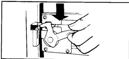
1. Push side of drawer closed, then latch the drawer side by pushing the latch up.
