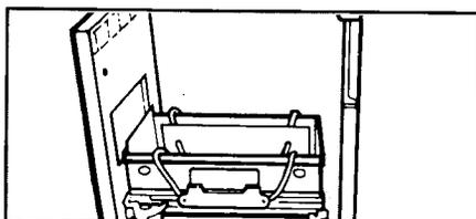
2. Fit the bag carrier in the drawer. Tuck the rope handles behind the bag retainers as shown.
