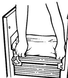
2. Lock bag in place by pulling the four prepunched holes over the bag retainer buttons. Holes will expand over the buttons without damaging the bag.
