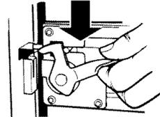
3. Hold the lever-action lock down and tilt the side of the drawer out until the lock clears the drawer front.
