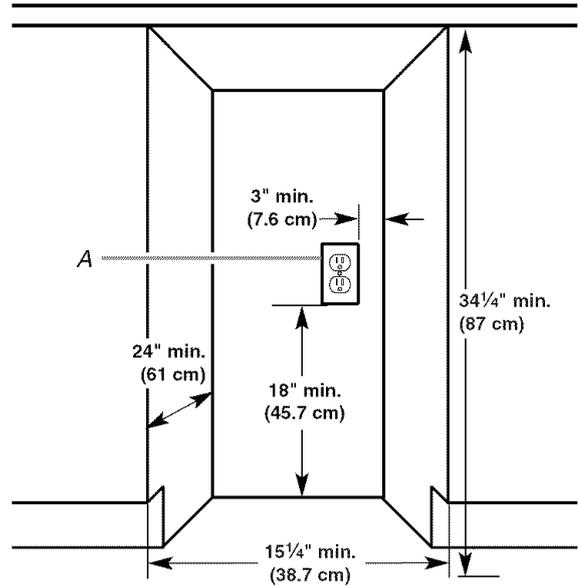
A. Grounded electrical outlet must be a minimum of 3" (7.6 cm) away from surrounding cabinets or nearby walls as shown. It can be placed either to the left or the right side of the compactor.
