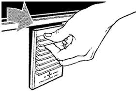
2. Remove the air filter by pulling the top edge of the filter. The filter should pull out easily. Throw away used filter.
