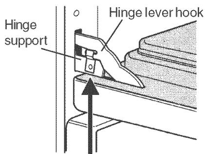
Lock engaged for door removal
