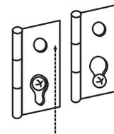
6. Close door and check that door strike aligns with door catch (B). If needed, slide door catch left or right within slot to adjust alignment.
