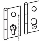
10. Remove door strike plug (B). Insert the door strike you removed in Step 8 in hole and secure with screw. Insert door strike plug in original door strike hole and secure with screw.
