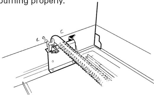
With the oven bottom removed, properly adjusted flames should have approximately 1" blue cones and, if range is supplied with natural gas, should burn with no yellow tipping. (With most LP gas, small yellow tips at the end of outer cones are normal.) Flames should not lift off burner ports. If lifting is observed, gradually reduce air shutter opening until flames are stabilized.
