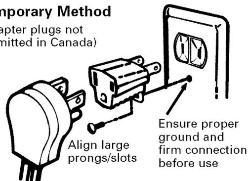
**CAUTION** — Attaching the adapter ground terminal to the wall receptacle cover screw does not ground the appliance unless the cover screw is metal, and not insulated, and the wall receptacle is grounded through the house wiring. The customer should have the circuit checked by a qualified electrician to make sure the receptacle is properly grounded.
