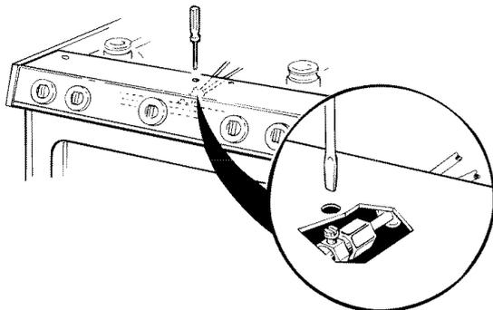
**CAUTION** — Make sure the surface burner control knobs are in the **OFF** position before attempting to adjust the pilots.
