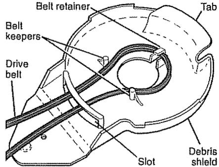
2. Route the other end of the new drive belt through hole in housing
