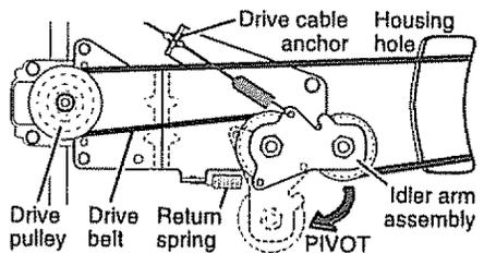
4. Pivot idler arm assembly to slacken drive belt, then remove drive belt from drive pulley, belt keepers and idler arm.
