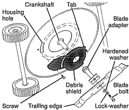
7. Use a wood block between blade and mower housing to prevent blade from turning when removing blade bolt.
