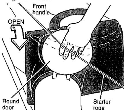
2. Remove grass catcher with clippings from lawn mower using both front and rear handles.
