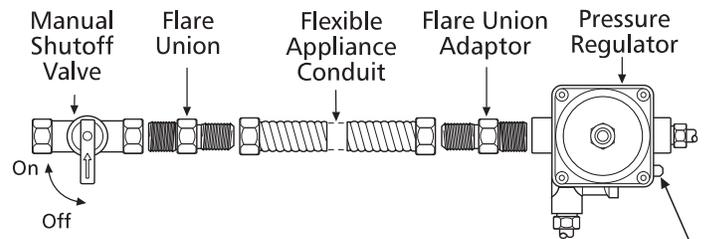
Service Shut-Off Valve Electric Ignition models only (Shown in ON Position). Be sure lever is in the "On" position when installation is complete
