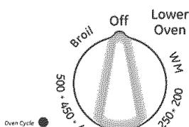
The Oven Cycle light glows until the oven reaches your selected temperature, then goes off and on with the oven element(s) during cooking.
