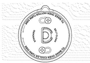
Turn the disk counterclockwise to increase the oven temperature.
