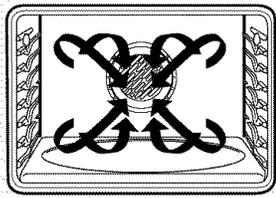
**NOTE:** The convection fan will cycle on and off while cooking to best distribute hot air in the oven.
