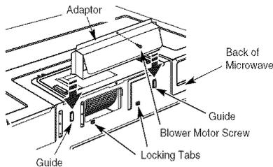
Push in securely until it is in the lower locking tabs. Take care to assure that the damper hinge is installed so that it is at the top and that the damper swings freely. Reinstall the original blower motor screw through the adaptor and into the back of the microwave.
