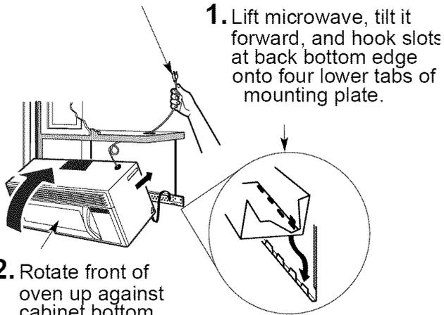
1. Lift microwave, tilt it forward, and hook slots at back bottom edge onto four lower tabs of mounting plate.
