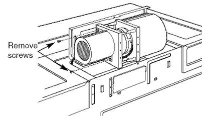
5. Roll the blower unit so that the right exhaust outlet faces the top. Snap the inlet sleeve back onto the left side with the opening facing down. **Note:** The left side sleeve opening must always face downward. Reinstall the 2 screws holding the inlet sleeve to the motor assembly.
