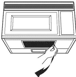
**7.** Install grease filter. See the Owner's Manual packed with the microwave oven.
