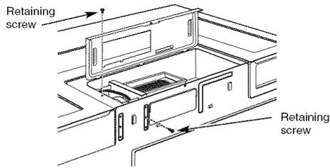
8. Close the blower cover and secure it with the screw removed in Step 1.
