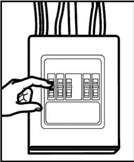
**CAUTION:** For personal safety, remove house fuse or open circuit breaker before beginning installation to avoid severe or fatal shock injury.
