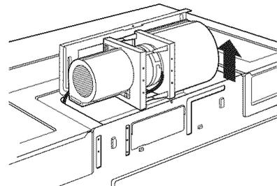
4. Remove the two screws holding the left side inlet sleeve to the blower unit. Snap the inlet sleeve off of the blower.
