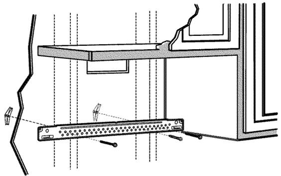
Attach the plate to the wall using toggle bolts. At least one wood screw must be used to attach the plate to the wall stud.
