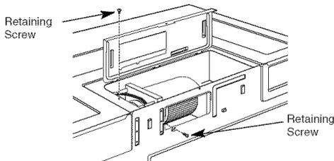
8. Close the blower cover and secure it with the screw removed in Step 1.
