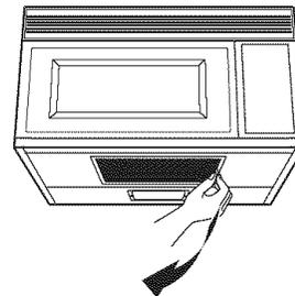
7. Install grease filter. See the Owner's Manual packed with the microwave.
