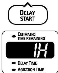
**STEP 5.** For a longer delay time, press DELAY START. The time will increase by one hour up to 9, 10, or 11 hours depending on your model.
