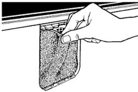
3. To replace air filter, push the replacement filter into place.
