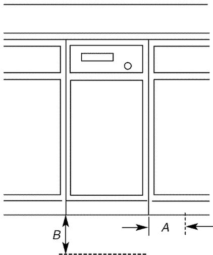
A. Leave 6" (15.2 cm) of clearance space to the right side of the compactor in order to remove the compactor bags.
