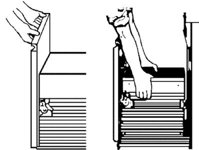
4. Place the other 2 corner posts on the floor to the side of the compactor. Grasp the sides of the compactor cabinet and put compactor on its side on top of the corner posts. Remove the shipping base from the bottom of the compactor.
