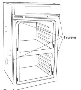
Important: Securely fasten oven to cabinet using the screws provided (two screws for a single oven or four screws for a double oven). Insert the screws through holes in mounting rails. Do Not overtighten screws.
