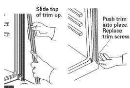
Slide top end of each trim upward onto oven side rails. Push each trim into place at bottom of trim. Use screws to attach each trim to oven. Take care not to scratch other surfaces with ends of trim.
