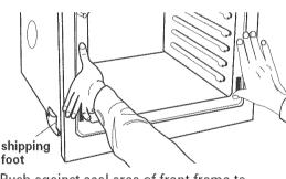
Push against seal area of front frame to push oven into cabinet until shipping feet almost contact cabinet. Use a Phillips screwdriver to remove screws attaching shipping feet. Remove and discard shipping feet.
