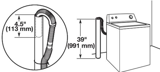
Minimum diameter for a standpipe drain: 2" (51 mm). Minimum carry-away capacity: 17 gal. (64 L) per minute. Some standpipes may require a Standpipe Adapter Kit and additional drain hose that may be purchased separately. See "Tools and Parts". Top of standpipe must be at least 39" (991 mm) high; install no higher than 96" (2.4 m) from bottom of washer. Installations higher than 96" (2.4 m) require a sump pump system.
