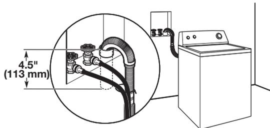
See requirements for floor standpipe drain system.
