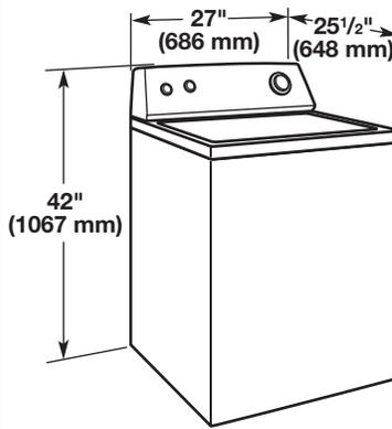
Select proper location for your washer to improve performance and minimize noise and possible "washer walk". Install your washer in a basement, laundry room, closet, or recessed area.
