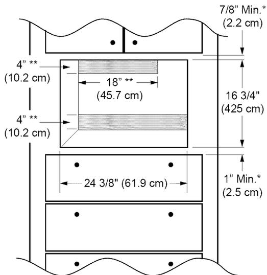
\* Minimum spacing: Includes additional space to avoid scraping/vibration.
