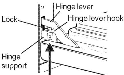
Lock engaged for door removal
