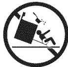
To reduce the risk of tipping, the range oven must be secured by properly installed anti-tip bracket(s) provided with the range. To check if the bracket(s) is installed properly, remove the lower panel or storage drawer and verify that the anti-tip bracket(s) is engaged. Refer to the Installation Instructions for proper anti-tip bracket(s) installation.
