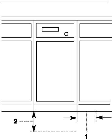
1. Leave 6 in. (15.2 cm) of clearance space to the right side of the compactor in order to remove the compactor bags.
