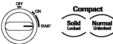
2. After 30 minutes or more, turn the Key-Knob to START to raise the compacting ram OR press NORMAL (UNLOCKED).
