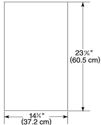
**Raised panel:** The outer section of panel must be  $\frac{7}{32}$  in. (5.6 mm) thick to fit into trim. Design raised panel sections using dimensions shown above.
