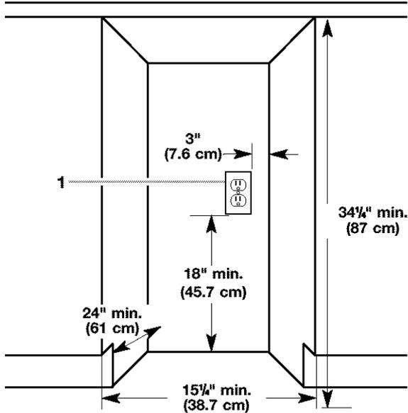
1. Grounded electrical outlet must be a minimum of 3 in. (7.6 cm) away from surrounding cabinets or nearby walls as shown. It can be placed either to the left or the right side of the product.
