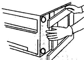
**4.** Place the other two corner posts on the floor to the side of compactor. Grasp sides of compactor cabinet and put compactor on its side on top of corner posts. Remove shipping base from bottom of compactor.
