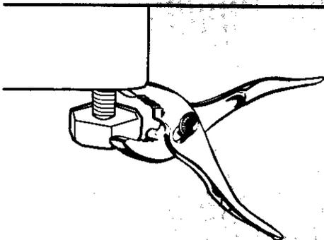
**6.** Use pliers to lower leveling legs away from cabinet. Adjust legs so there will be 1/8" (3 mm) to 1/4" (6.4 mm) space between top of compactor and top of cabinet opening. Stand compactor upright.
