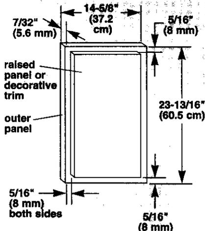
**Raised panel:** The outer section of panel must be 7/32" (5.6 mm) thick to fit into trim. Raised decorative trim or raised panel sections must be 5/16" (8 mm) from the side, bottom, and top edges of outer section.
