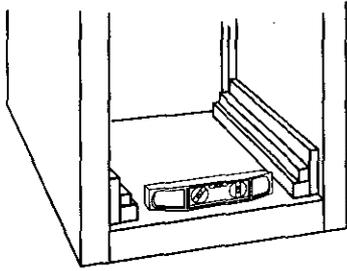
**7.** Place level inside on floor of cabinet. Check that compactor is level from front to back and side to side. Adjust leveling legs until compactor is level.
