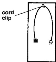
**2.** Check that power supply cord is attached to the cord clip on the rear of compactor.
