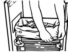
3. Push Side-Lock Latch down and tilt drawer side open.
