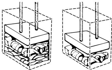
Load bulky trash, bottles, and cans in the center of the drawer. Bottles or cans not placed in the center may become caught between the ram and the drawer. The Drawer Monitor Switch then senses a "misload" and causes the ram to return to the "up" position without compacting.
