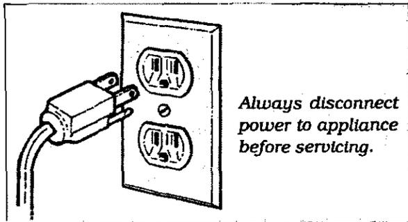
If an ungrounded, two-hole or other type electrical outlet is encountered, it is the **personal responsibility of the appliance owner to have the receptacle replaced with a properly grounded three-hole electrical outlet**. The three-prong grounding plug is provided for protection against shock hazards. **Do not cut or remove the third grounding prong from the power cord plug.**
