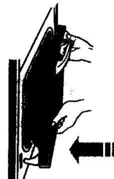
2. Open the door completely and remove the door removal pins. Save them for future use.
