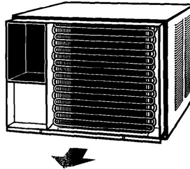
5. Install the drain plug and drain cup (accessory parts) to rear of cabinet. Slide drain cup down into rear support between grooves in cup.
