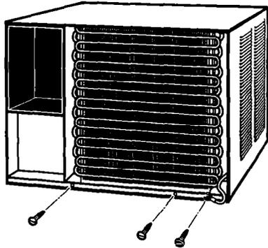
3. Remove the rear shipping screws (2).
